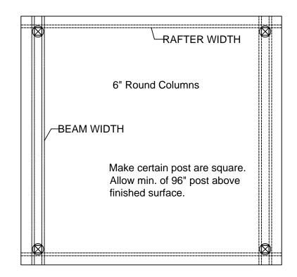
STEP #1 POST SPACING - All Spacing will be Outside of Post to Outside of Post.
